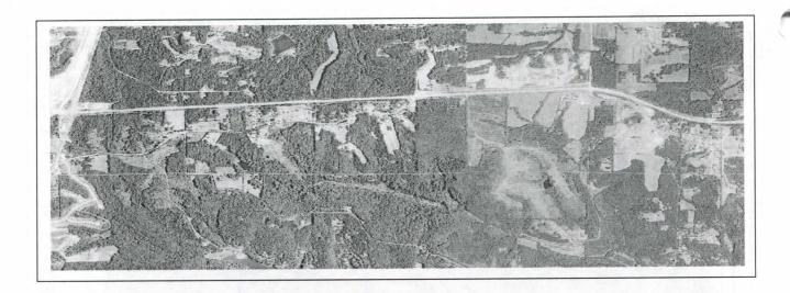
In this view New A Highway can be seen as the major line in the north half running east and west. Note the thin line below A Highway, paralleling it, this is the "New Road" it follows the Township line across the county. Pioneer, or Old Highway A, can be seen as the squiggly line between the two in the left half.
